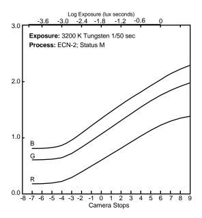
The curves describe this film's response to red, green, and blue light. Sensitometric curves determine the change in density on the film for a given change in log exposure.<sup>1</sup>
